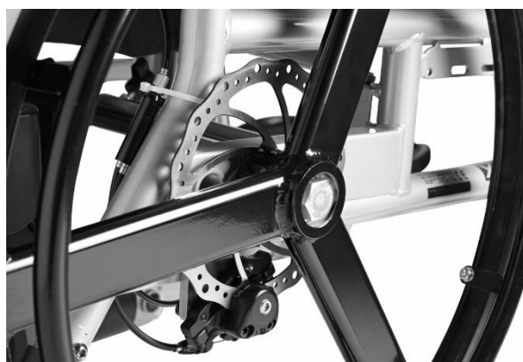
Minimaxx wheelchair with disc brakes.
